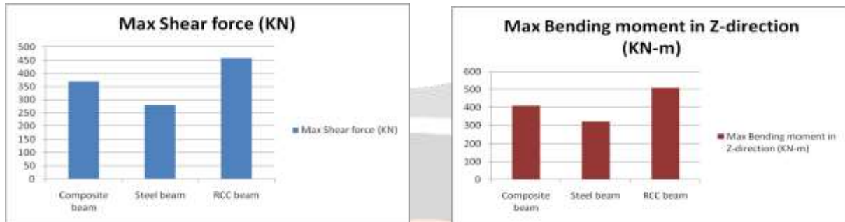
Fig-10: Max shear force and Max Bending Moment for RCC Steel and composite structure
