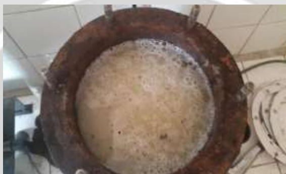
Photo 9: Loading must into the distiller
