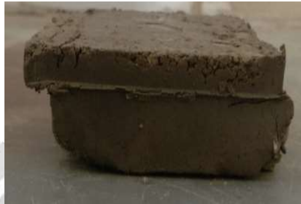
Fig.-3 Tested soil sample of DST ( Rc 90% )
