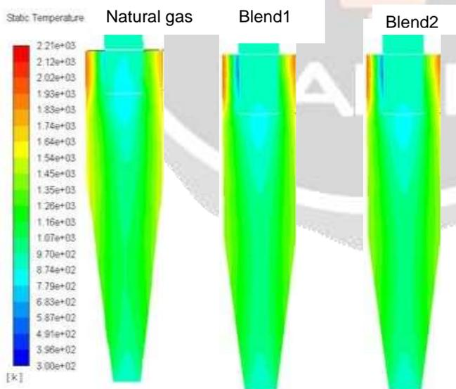
Figure 3: Temperature profiles inside the furnace obtained from 3 simulation cases
