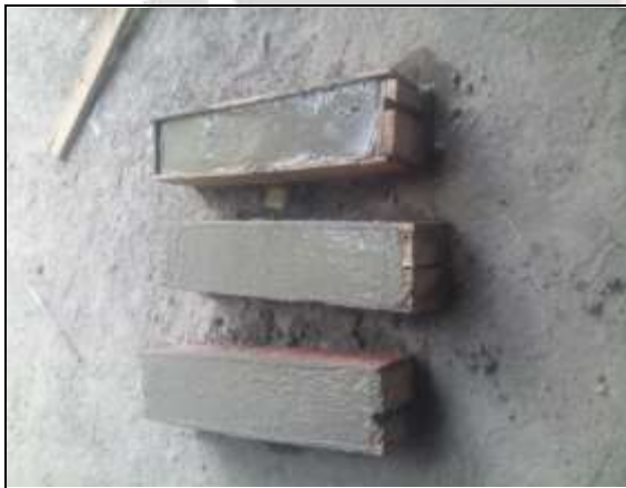
Fig -1: Casting of beams
