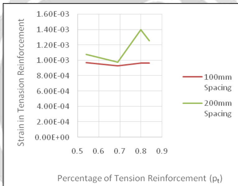
Chart-5. Strain in Tension Reinforcement for all models
