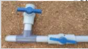
Fig 16: T-Joint and Ball Valve
