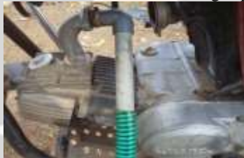
Fig 17: Connecting Wood Gas to the Engine
