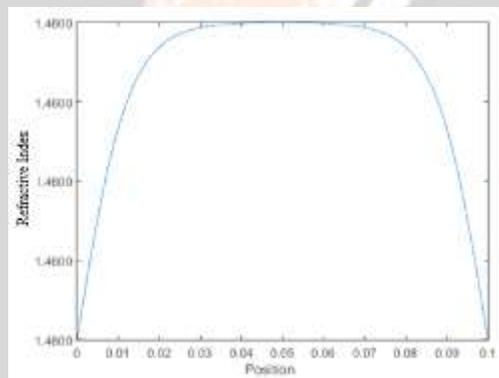
**Fig -11:** The refractive index as a function of the position of the grating
