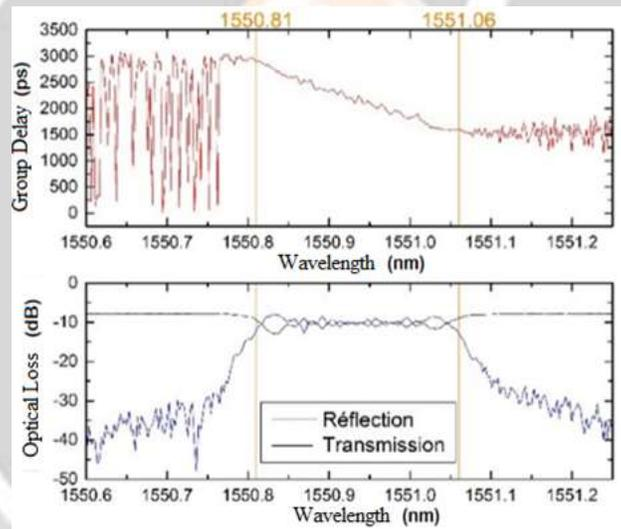
**Fig -16:** Delay and reflection time of an RDB on a 15 cm long- fiber and with a step of 0.0125 nm / cm
