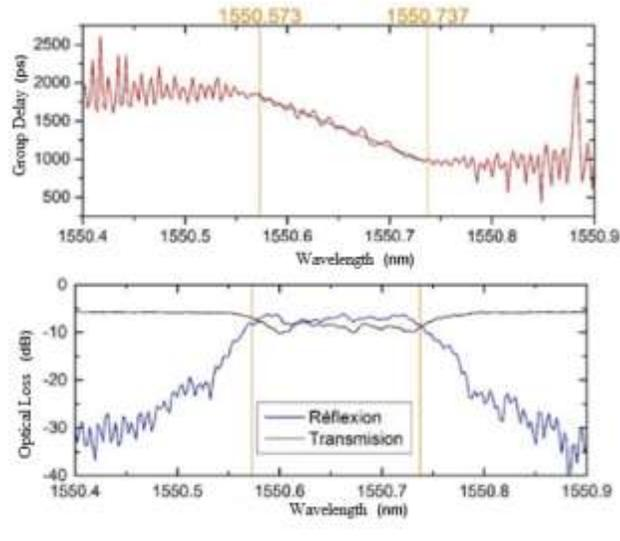
**Fig -15:** Delay and reflection time of an RDB on a 10cm- long fiber and with a step of 0.0125 nm / cm
