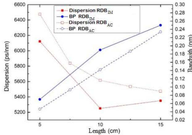
**Fig -17:** Evolution of dispersion and current bandwidth for improved RDBs with a step of 0.0125 nm / cm and lengths varying from 5 to 15 cm
