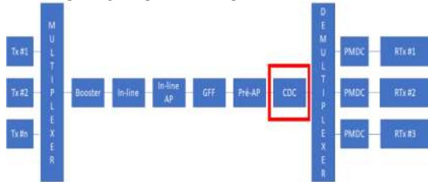
**Fig -4:** Block diagram of an optical link in a 5G network
