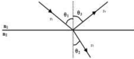
**Fig -12:** Illustration of refractive index in an optical fiber
