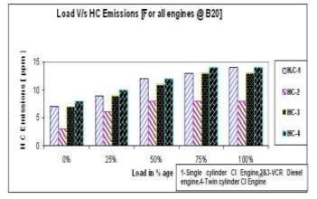
It is observed that slight variations of NOx emissions occur in all engines at 0% load and 100% load conditions; the reason for these variations could be malfunctioning of biofuel mixture. From the results it is observed that lower (30-50%) hydrocarbon emissions occur in the case of VCR engine at 18:1 CR compared to single cylinder and twin cylinder engines. The reason for this could be incomplete combustion and physical properties of the CBF.
