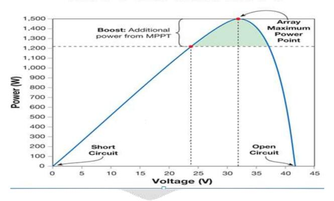
So the readings shows by maximum power point tracking **24.77** % of efficiency increases. So this could be the most economical solution for better performance of plant.
