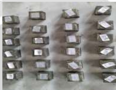
Fig 15: Cement mortar cubes
