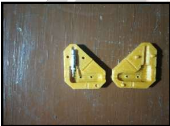
Fig5.4: Inserted Audio jack for outer covering and casting
