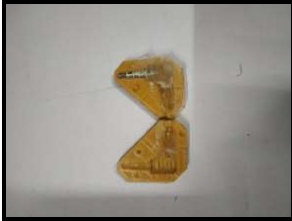
Fig5.5: Opening The 3D printed Mould after 5 minutes of cooling
