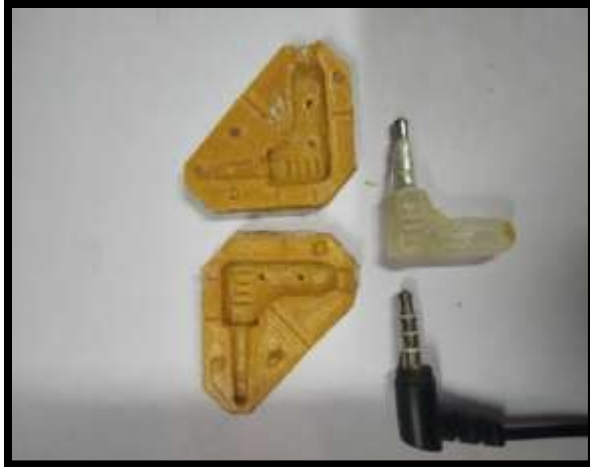
Fig5.7 : Observation Comparison Between 3D Printed Mould cast and Industrial Mould Cast
