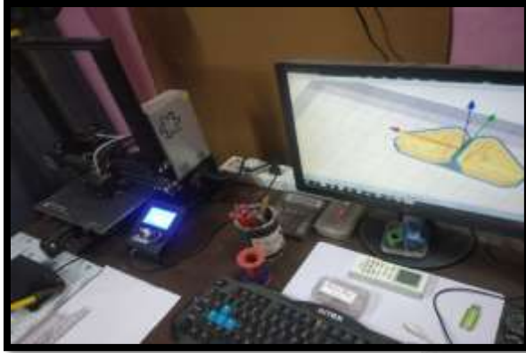
Fig5.1 :Mould making in 3D printer with Software Ultimaker Cura
