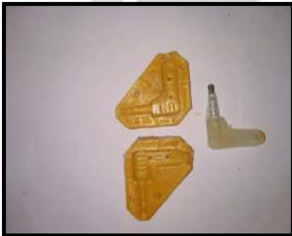
Fig5.6: Taking Out The cast From 3D printed Mould
