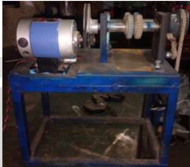
Fig -6 Nylon Spur gear with and without Phasing arrangement
