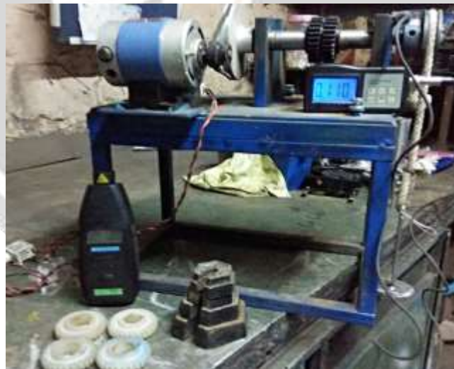
Fig -7 ABS Polymer Integrated and non-integrated phased Spur gear arrangement
