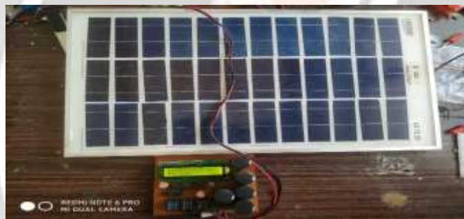
Fig. 2: Actual hardware model of capacitor with battery to optimize the performance of PV System
