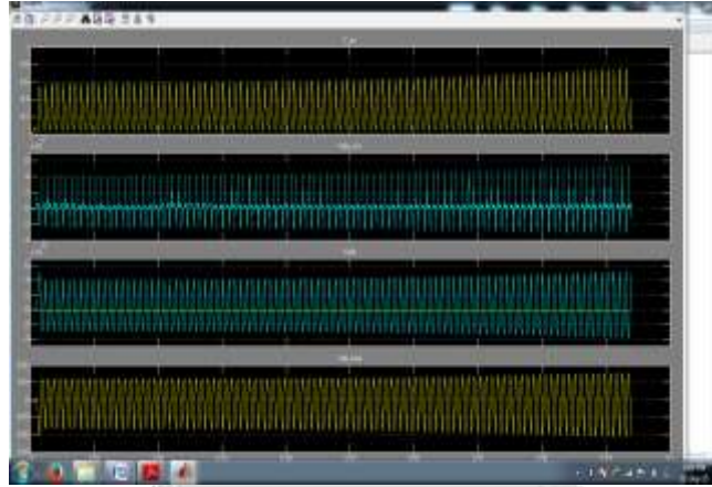
Fig .7. Wind turbine power inverter waveform.
