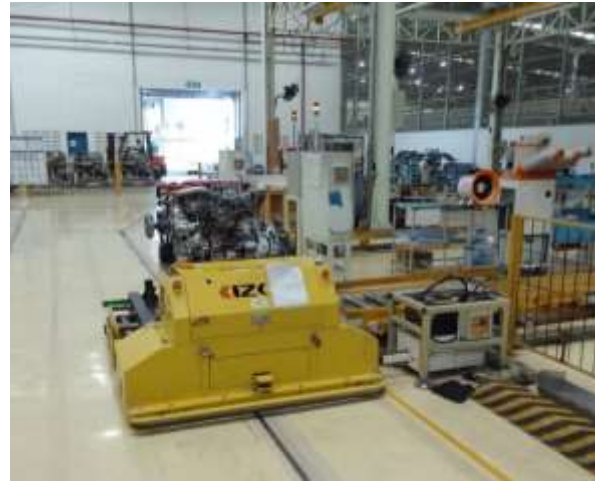
Fig- 6 AGV Delivers Engine After Test to Qualified Station
