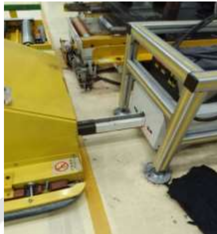
Fig- 2 Battery Charging Process on AGV
