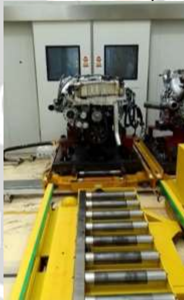
Fig- 5 AGV Delivers Engine Before Test to Testbench
