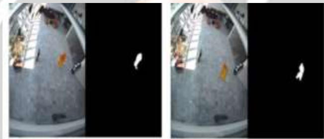
Fig.4. Illustration of blob's aspect ratio related to faint detection
