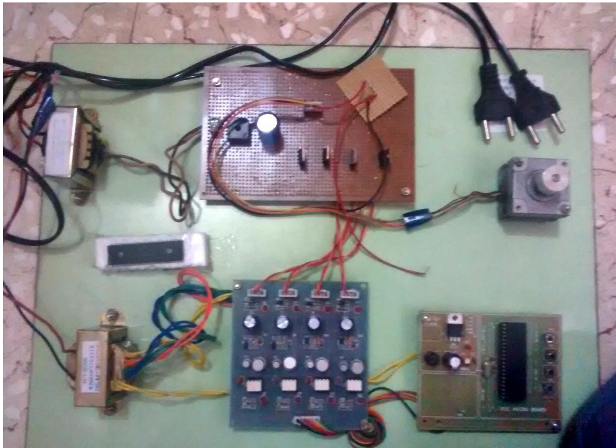
Fig 2:-Hardware set-up for driving the Hybrid stepper motor for full step excitation mode under no load.
