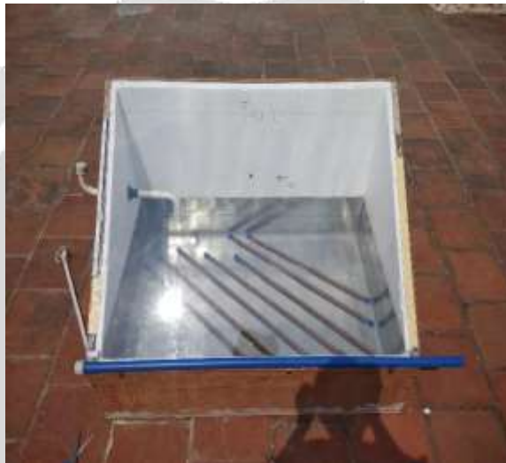
Fig.-2.1: Solar still with PCM material
