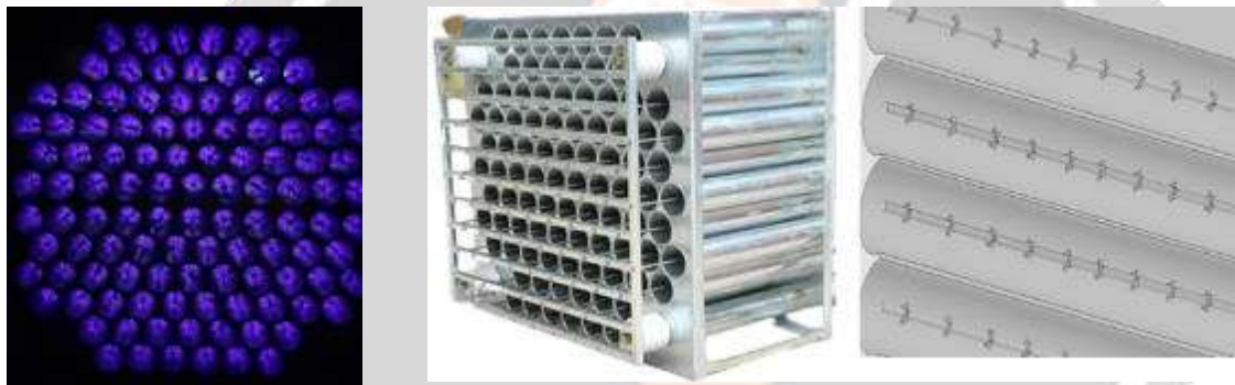
Fig - 4: Structure of Electrostatic precipitation
