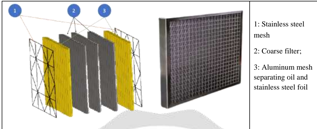
Fig - 3: 7-layer oil separator dust collector filter
