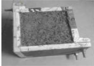
Figure 8. The mixture is properly compacted into the mould
