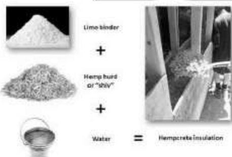
Figure 2. Constituent raw materials
