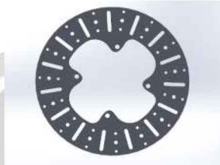
Chart -1: Drilled & slotted disc rotor profile
