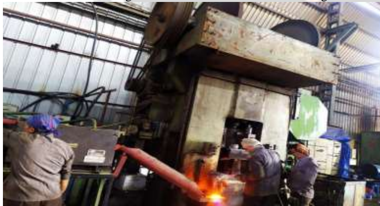
Fig Mechanical screw press with automated induction heating arrangement
