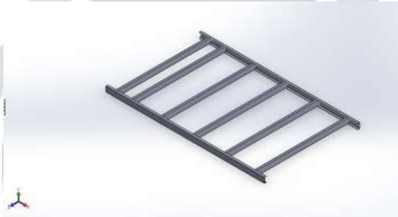
Figure 1 SolidWorks model of C – c/s ladder chassis
