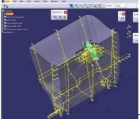
The process being described involves creating a section view of a glove box using a master
