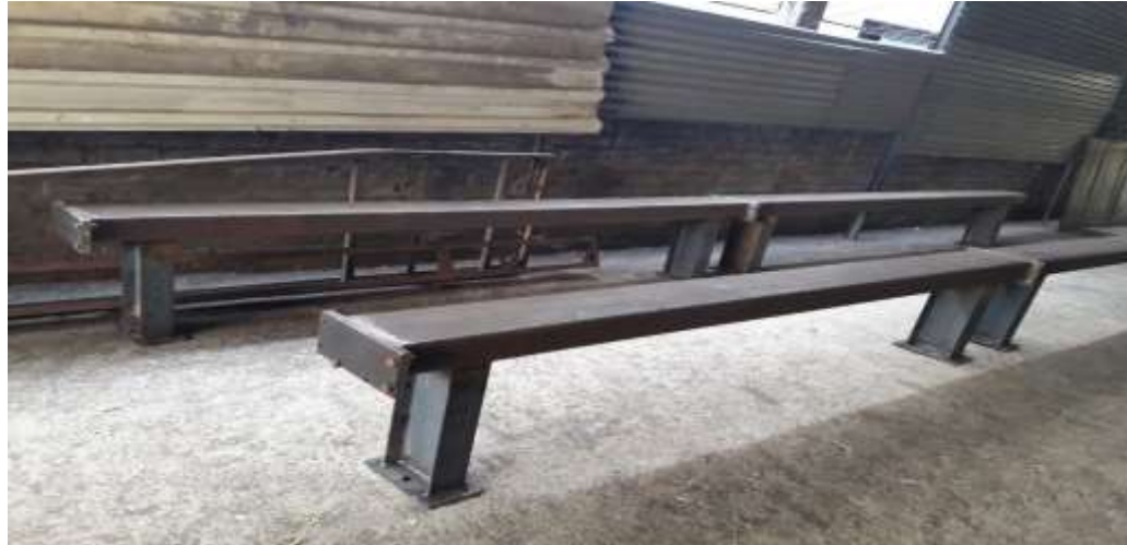
Fig 4.1 Base of plasma cutting machine (Omega CNC Automation)
