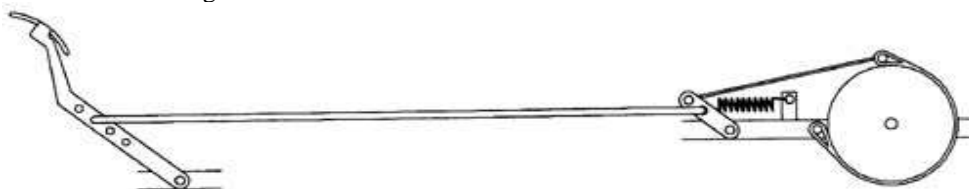
BRAKE ON Fig 8: Braking Mechanism
