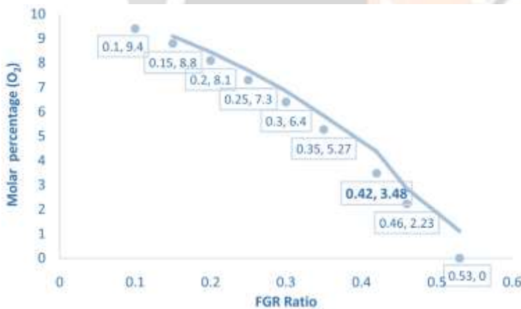
Figure 5. FGR ratio effects on O 2 concentration in exhaust gas.
