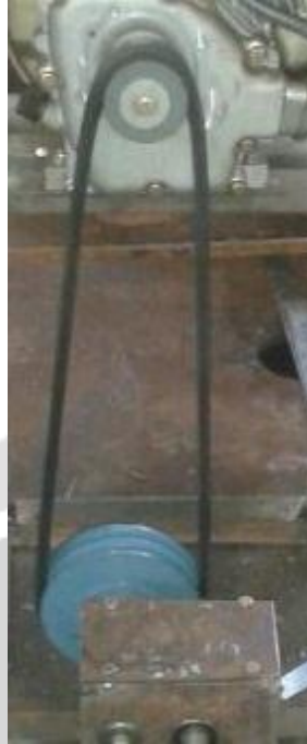
Fig. 7: Belt drive (drive from engine to spur gearbox)
