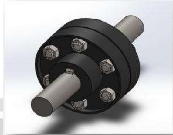
Fig. 2: Isometric view of CAD model of bushed pin flexible coupling
