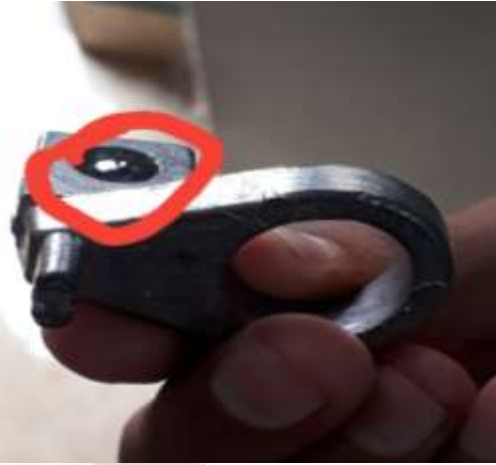
Fig.5 External blow holes
