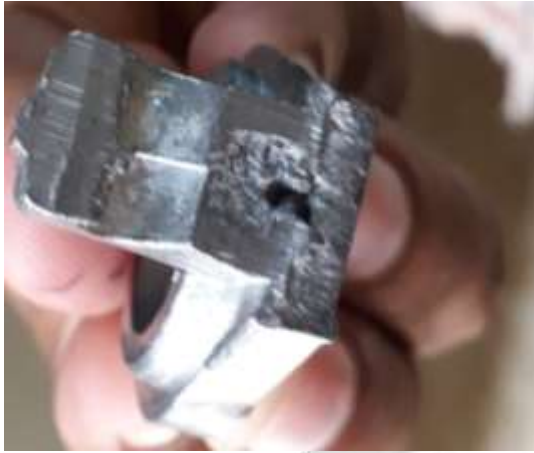
Fig.4 Internal blow holes in component
