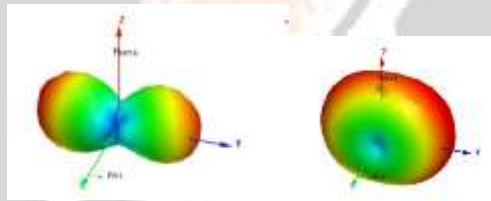
Figure 2 The simulated radiation patters of the 1-D 10-element smart antennasystem.
