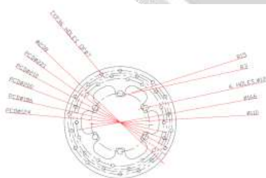
Fig. 5.1 2D Sketch of Conventional Brake Disc
