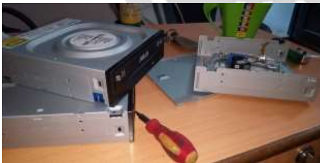
Fig. 2: Disassembly of Optical Drives
