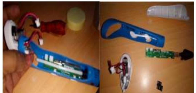
Fig. 5: Disassembly of 3D Pen
