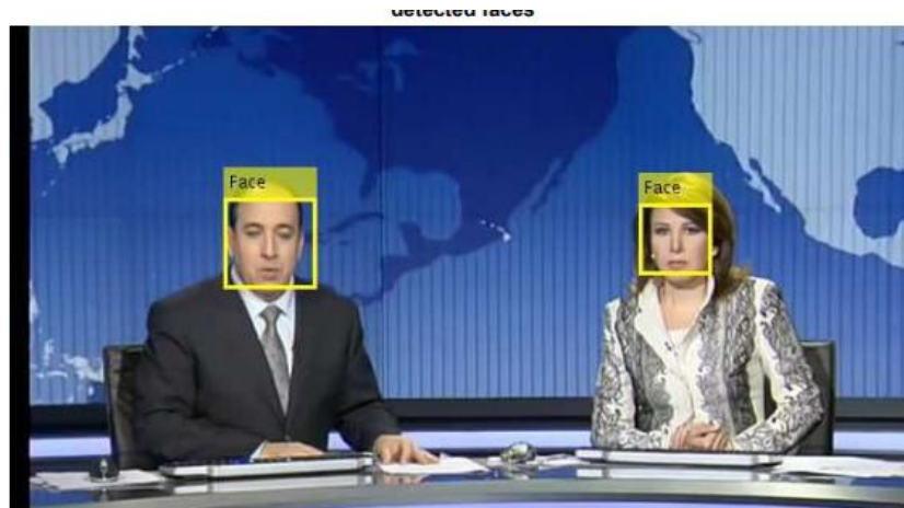
Figure 5: An example to represent the output of Viola-Jones face detection algorithm. scales slide across the granted frame and infusion Haar features. These extracted Haar characteristic are passed to Waterfall classifier for detection of face.
