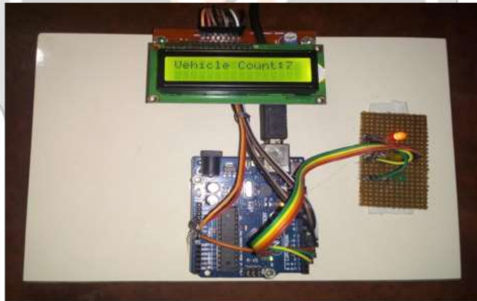
Fig- 16 Red light glows when the count becomes greater than the threshold value
