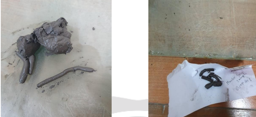
Fig 5 – Plastic limit test
