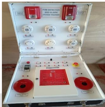
Figure 2: The developed Fire Detection and Alarm System Trainer in an Open Position
