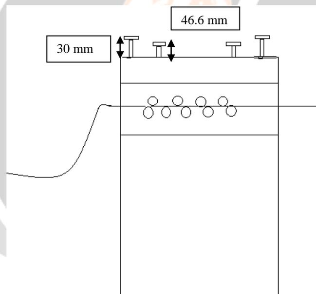
**Fig 5:-** length of bolts after tightening or post tightening position of bolts
