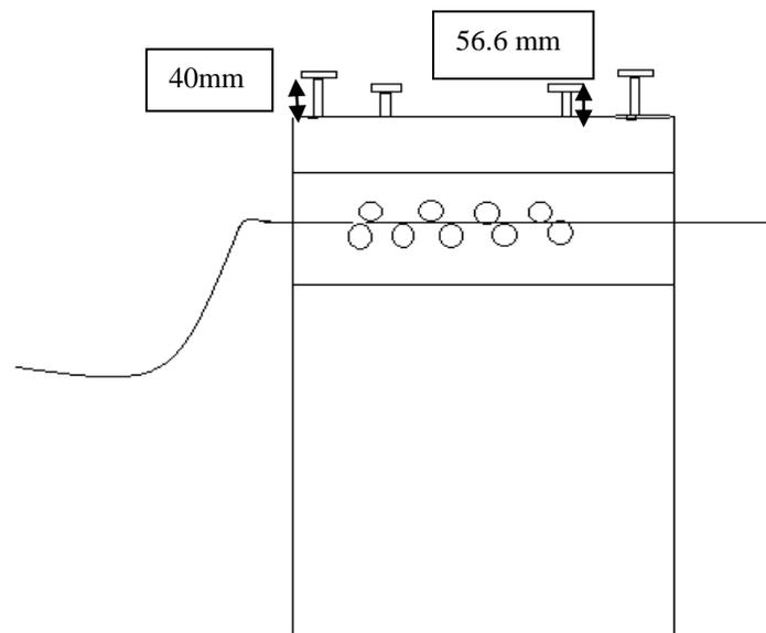
**Fig 4:-** height of bolts before tightening or initial position of bolts
