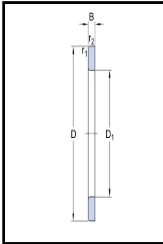
**Fig 1:-** General drawing of washer<sup>[12]</sup>
