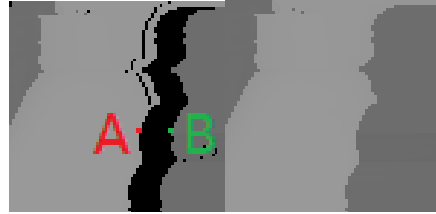
Fig. 2: (a) Warped depth map; (b) Filled depth map using depth based extrapolation [2]
