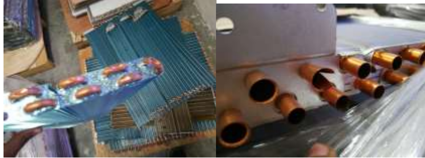
Fig.1 Cracked or Damaged tube.
