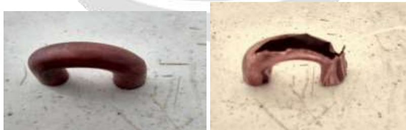
Fig.5.2 Before and after when reacted with nitric acid.
