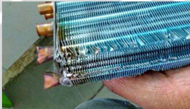
Fig.5.1 Damaged heat exchanger due to heating.
