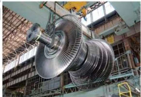
Fig. 1 Actual View of Low Pressure Turbine
