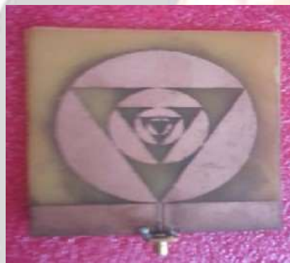
Fig -2: Fractal antenna views in front side with four iterations
