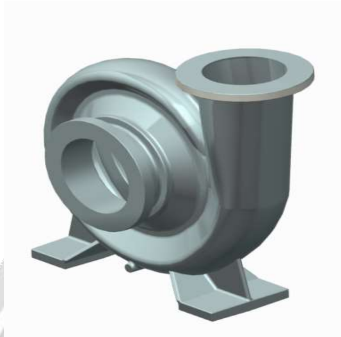
Fig no.3: 3D model for Casing
