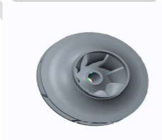
Fig no.2: 3D Model of Impeller
