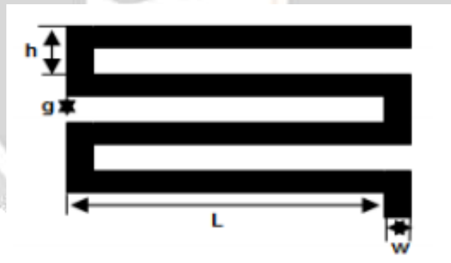
Fig -1: Meandered shape with dimensions
