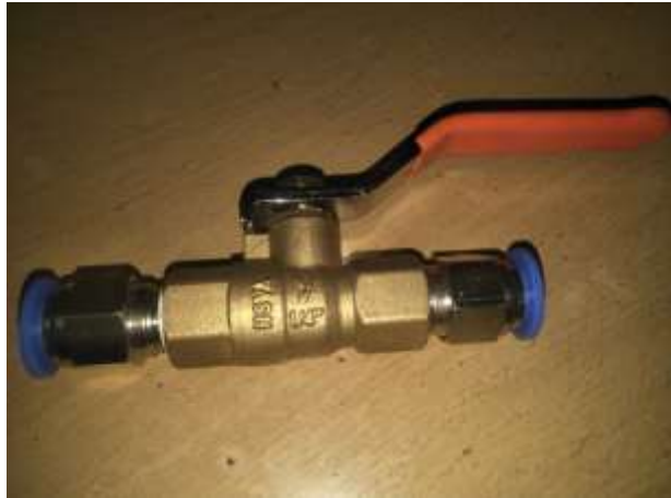
Fig. 8: Flow control valve
