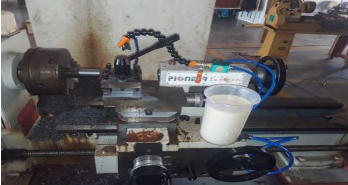
Fig.12: Attachment of SQL cooling system setup with machine
