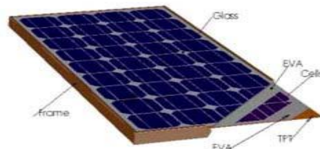
Figure 1: typical schematic diagram of the solarmodule
