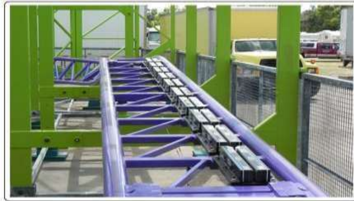
Fig.3 Roller coasters with an electromagnet
