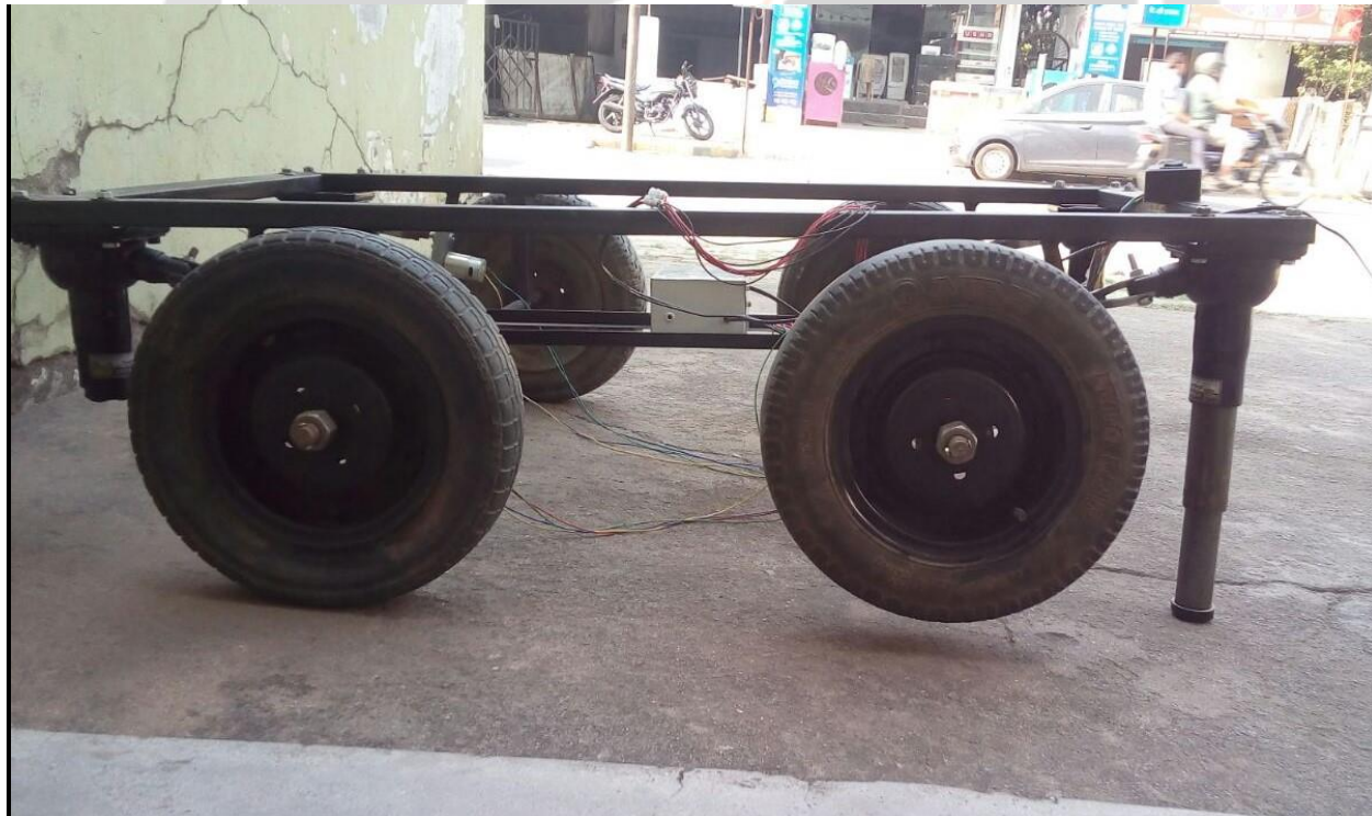
Fig-5: Side view of vehicle when front right wheel of vehicle is lifted
