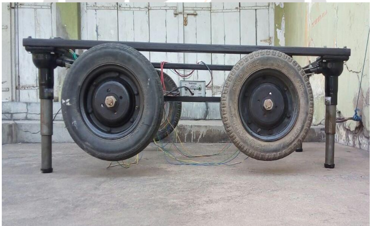
Fig-7: Side view of vehicle when all 4 wheels are lifted
