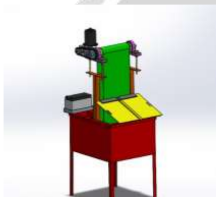
Fig 2. 3D SolidWorks Model of Oil Skimmer
