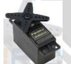
This high-torque standard servo can rotate approximately 180 degrees (90 in each direction). It has inbuilt gear & feedback mechanism to perform control action. The S3003 180 Degree Rotation Servo Motor rotates 90° in each direction making it 180° servo motor. It is a Digital Servo Motor which receives and processes PWM signal faster and better. It equips sophisticated internal circuitry that provides good torque,
